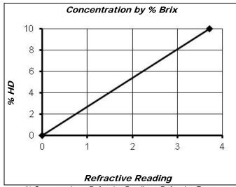
% Concentration = Refractive Reading x Refractive Factor Coolant Refractometer Factor % Brix = 2.7
