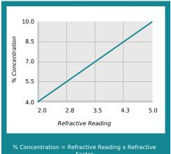
Factor Coolant Refractometer Factor % Brix = 2.0
