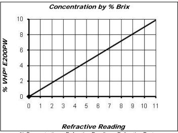
% Concentration = Refractive Reading x Refractive Factor Coolant Refractometer Factor % Brix = 0.9
