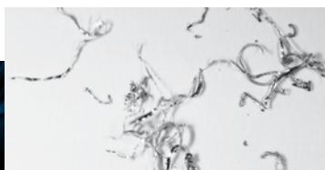
Metal shavings from Tiger Aluminum disc.
