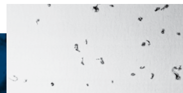
Metal shavings from a conventional disc.
