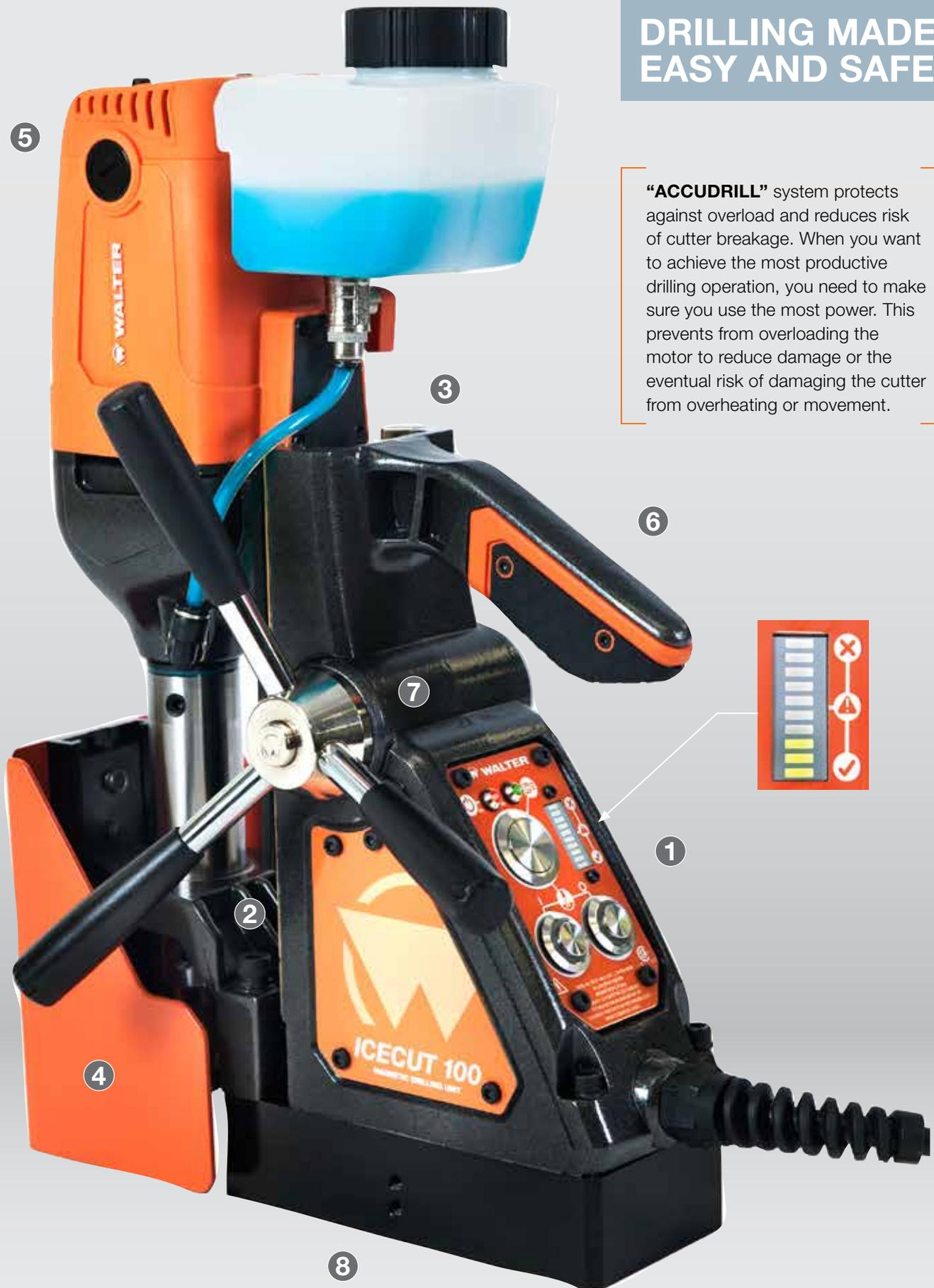
“**ACCUDRILL**” system protects against overload and reduces risk of cutter breakage. When you want to achieve the most productive drilling operation, you need to make sure you use the most power. This prevents from overloading the motor to reduce damage or the eventual risk of damaging the cutter from overheating or movement.
