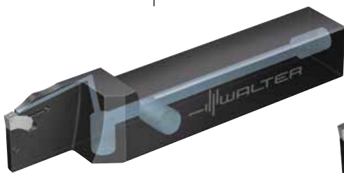
G2012-P Monoblock toolholder with precise internal coolant supply, parting off up to a diameter of 90 mm
