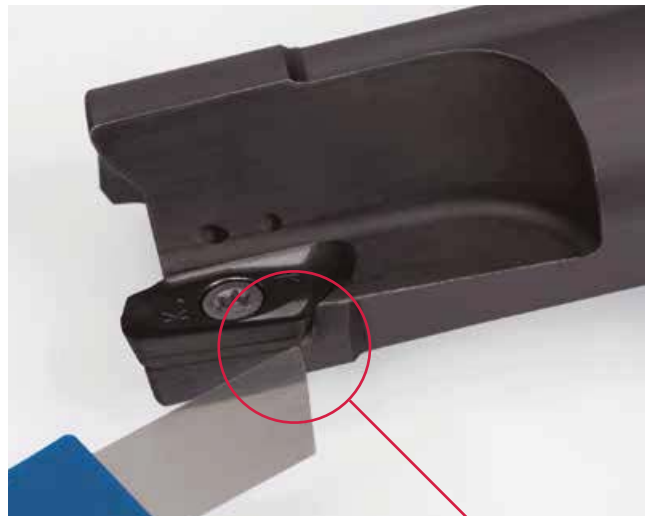
Check with 0.01 mm spacer
