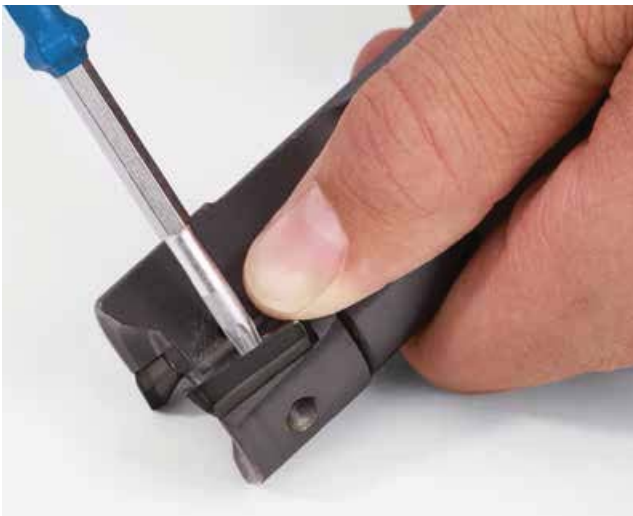
Apply pressure to the rear part of the indexable insert when tightening
