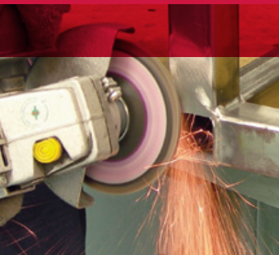
Grinding welds on a fabricated Steel part.
