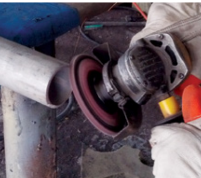
Grinding and beveling Stainless Steel tubing a with a Saber Tooth abrasive flap disc.
