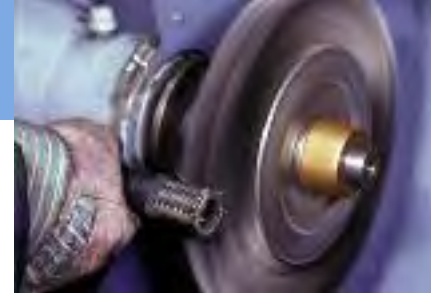
Removing rubber coating from a hydraulic hose.
