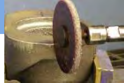
Removing casting flash from ductile-iron housing with an encapsulated brush.
