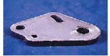
Blanked steel part before deburring.
