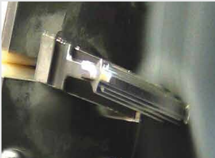
Nylox brushes can be used to produce large edge radii on turbine blades. Robotic manipulation of the part provides a high degree of uniformity and good control of radius size. Using this type of process, edge radii of more than .020" can be produced.
