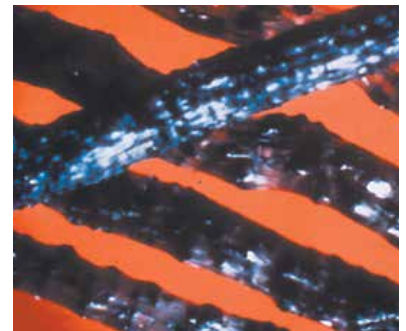
A magnified view of Nylox filaments shows the abrasive grains which are impregnated in the nylon carrier. During operation, burrs are removed by an abrading action in which filaments act like files. Unlike wire brushes, Nylox brushes need to be run at low speeds and significant pressures for maximum effectiveness.
