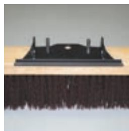
Flip scraper and place over bolts
