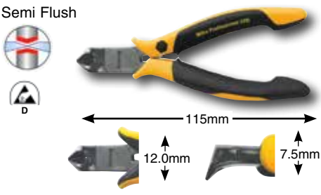
32726 Oblique Angled Cutters, 29°, Short Head, Semi Flush
