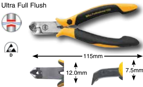
32724 Oblique Angled Cutters, 29°, Full Flush
