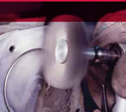
Removing carbon build-up from an engine.
