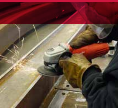
Smoothing the edges of roller coaster track with a resin fiber disc.
