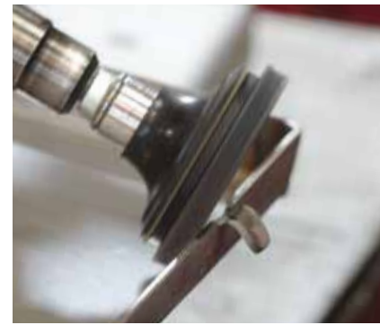
Edge chamfering a fabricated stainless component.
