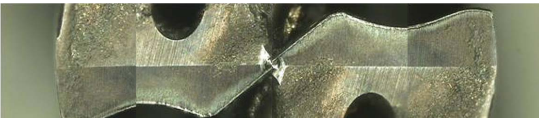
Competitor A (After Drilling 546 Holes)
