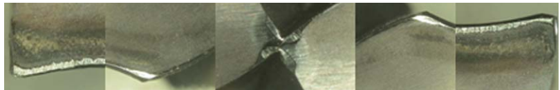
YG-1 (Total Drilling 600 Holes)
