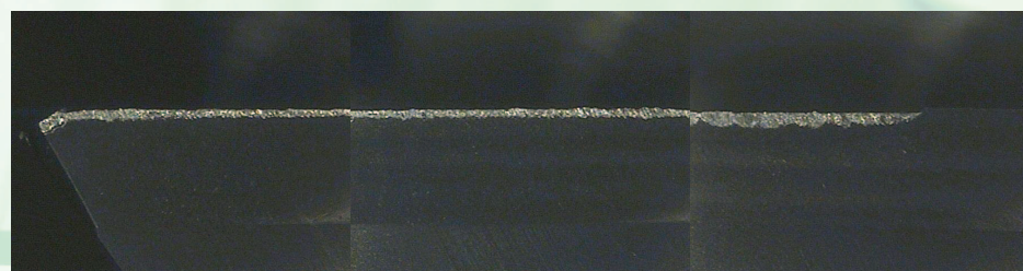
YG-1 V7 STEEL (Total Milling Length 10m)
