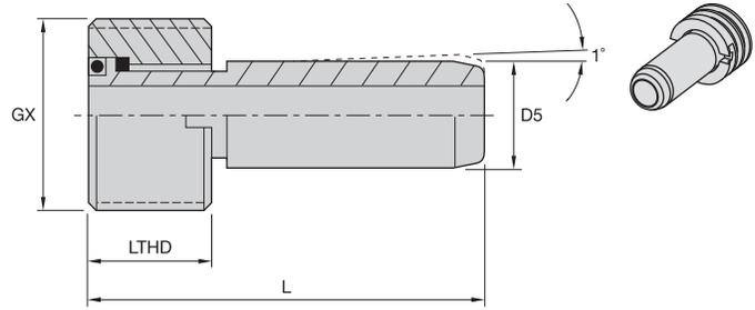
■ HSK Coolant Supply Unit • Assembly
