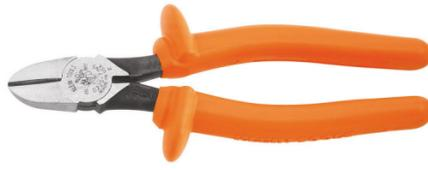
These Insulated Diagonal-Cutting pliers have dual layered grips that are flame retardant, impact resistant, and rated for 1000-volts. They feature a heavy-duty tapered nose design with induction hardened cutting knives for durability. They are made of forged steel and have a hot-riveted joint for smooth action and no handle wobble.
