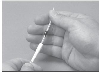
7.8 Place the strain relief boot and clear strain relief tube/crimp ring assembly on the buffered fiber.
