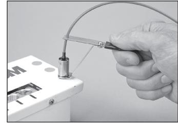
8.21 Rest the connector holder in one of the available cooling ports located on both sides of the oven. Let cool for three minutes.
