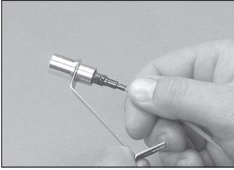
9.1 Remove the 3M™ Hot Melt Connector from the 3M™ Universal Connector Holder if necessary.
