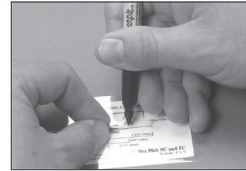
7.9 Place the buffered fiber on the strip template for "FC Hot Melt" and use the fiber marking pen to mark the location of the buffer cut.
