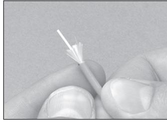
6.14 Flare the Kevlar® fibers equally around the buffered fiber.
