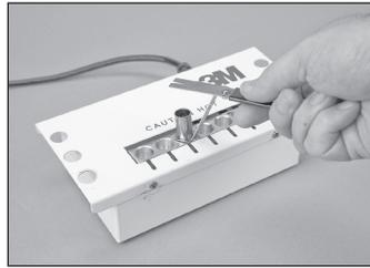
7.5 Place the connector holder into an available port in the oven.
