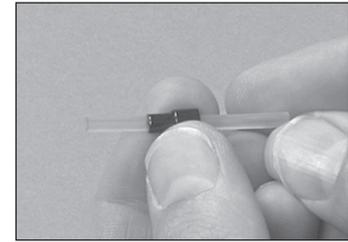
7.6 Insert the clear strain relief tube into the metal crimp ring until the end of the tube is positioned in the small half of the crimp ring.
