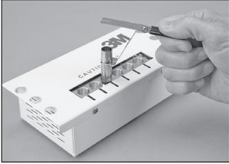
4.16 Remove the 3M™ Universal Connector Holder from the 3M Hot Melt Oven by grasping the cool-touch handle.
