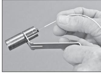
3.14 Feed the fiber into the back of the 3M Hot Melt ST Connector, until the buffer stops inside the connector.
