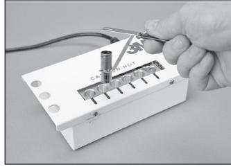
5.14 Remove the 3M™ Universal Connector Holder from the 3M Hot Melt Oven by grasping the cool-touch handle.
