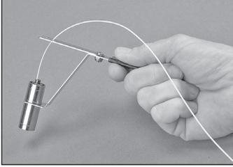
3.16 Push the buffered fiber into the cable retention feature until secure.
