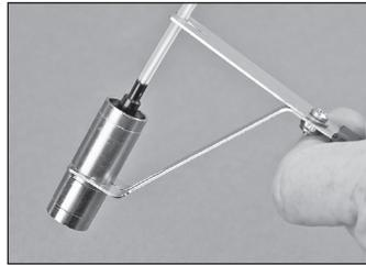
7.17 Push the buffered fiber into the cable retention feature until secure.
