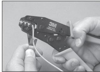
8.23 Secure the small portion of the crimp ring onto the jacket with the die labeled .137.
