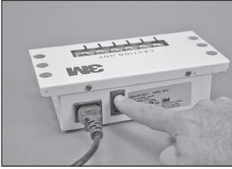
7.1 Plug in the 120V or 230V power cord. Turn on the 3M™ Hot Melt Oven. The oven requires six minutes to warm up.
