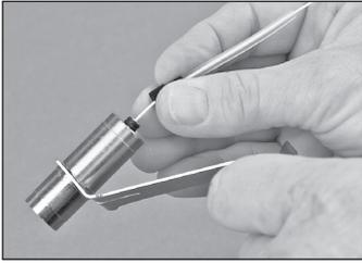
5.16 Slide the metal crimp ring assembly onto the back of the connector.
