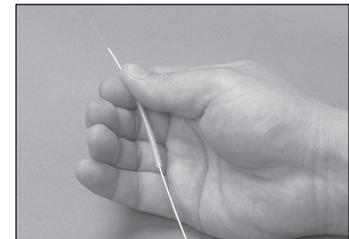
3.12 Position the clear strain relief tubing towards the end of the fiber where it will be easily accessible.
