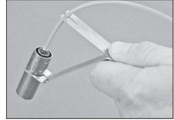
4.18 Push the jacketed fiber into the cable retention feature keeping the fiber as straight as possible.
