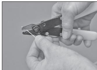
7.11 Using the 3M™ Stripping Tool 6362-TH, remove the buffer in small pieces until 9/16" (14 mm) of buffer has been removed.
