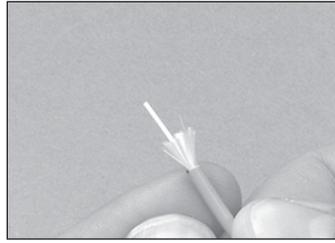
8.14 Flare the Kevlar® fibers equally around the buffered fiber.
