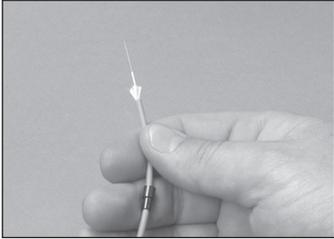
6.16 Position the metal crimp ring towards the end of the cable where it will be easily accessible.
