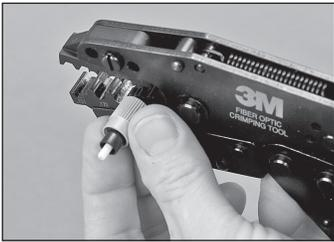
8.22 Once connector has cooled, remove from connector holder. Using the die labeled .190, crimp the large portion of the crimp ring onto the connector.
