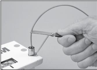
4.19 Rest the connector holder in one of the available cooling ports located on both sides of the oven. Let cool for three minutes.
