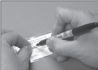
3.7 Place the buffered fiber on the strip template for "ST Hot Melt" and use the fiber marking pen to mark the location of the buffer cut.
