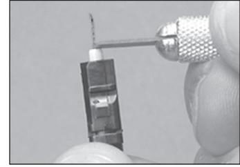
9.3 Position the scribe blade so the flat side of the blade is resting on the bead of adhesive and the blade is perpendicular to the fiber.
