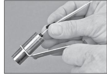
7.15 Feed the fiber into the back of the 3M Hot Melt Connector, until the buffer stops inside the connector.
