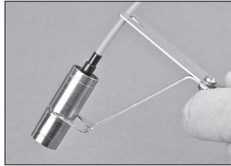
8.20 Push the jacketed fiber into the cable retention feature until secure.
