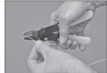
3.9 Using the 3M™ Stripping Tool 6362-TH, remove the buffer in small pieces until 7/8" (22 mm) of buffer has been removed.
