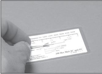
7.13 Check the final strip lengths and adjust if necessary.
