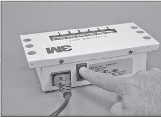
3.1 Plug in the 120V or 230V power cord. Turn on the 3M™ Hot Melt Oven. The oven requires six minutes to warm up.
