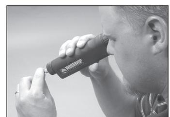
11.21 Inspect the connector endface with the fiber through coaxial and oblique views by changing the view with the thumbswitch on the body of the 3M View Scope.
