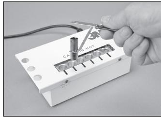
7.14 Remove the 3M™ Universal Connector Holder from the Hot Melt Oven by grasping the cool-touch handle.
