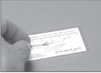
5.13 Check the final strip lengths and adjust if necessary.
