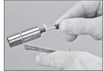
6.18 Feed the fiber into the back of the 3M Hot Melt Connector, pushing until the jacket stops on the connector. Flare the Kevlar® fibers equally around the buffered fiber.
