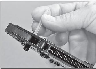
7.7 Using the die labeled .137, crimp the small half of the crimp ring to the clear strain relief tubing.
