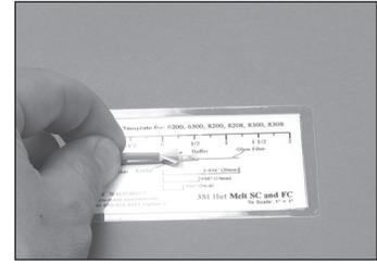
8.15 Check the final strip lengths and adjust if necessary.
