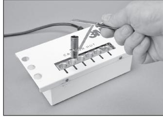
8.17 Remove the 3M™ Universal Connector Holder from the 3M Hot Melt Oven by grasping the cool-touch handle.
