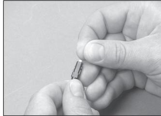
9.5 Pull the fiber away from the connector. Pull along the axis of the fiber, not to one side or the other. If the fiber does not break away, score the fiber again.
