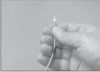
8.16 Position the metal crimp ring towards the end of the cable where it will be easily accessible.
