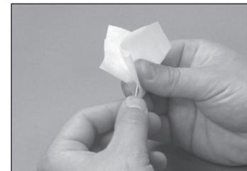
7.12 Using a lint free cloth moistened with Isopropyl alcohol, clean the bare fiber to remove any oils or Acrylate coating debris.
