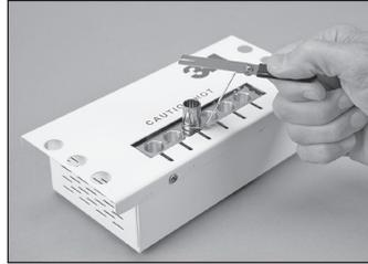
3.5 Place the connector holder into an available port in the oven.
