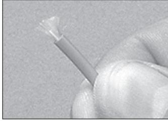
4.14 Flare the Kevlar® fibers equally around the buffered fiber.
