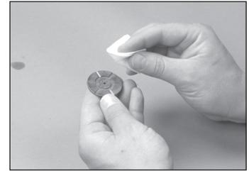
11.15 Clean the flat side of the 3M Polishing Jig with a lint free cloth moistened with Isopropyl alcohol.
