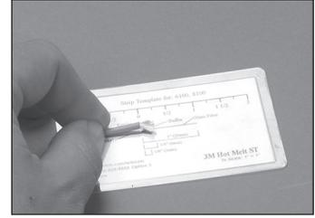
4.15 Check the final strip lengths and adjust if necessary.
