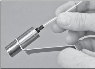
7.16 Slide the clear strain relief tube/crimping assembly to the connector until it stops.
