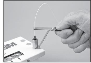
5.18 Rest the connector holder in one of the available cooling ports located on both sides of the oven. Let cool for three minutes.
