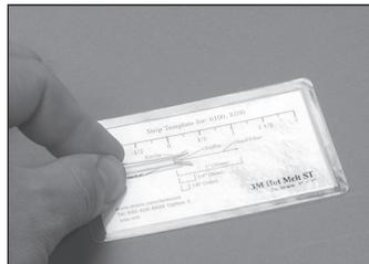
3.11 Check the final strip lengths and adjust if necessary.
