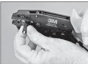
6.22 Once connector has cooled, remove from connector holder. Using the die labeled .190, crimp the large portion of the crimp ring onto the connector.
