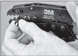
5.19 Once connector has cooled, remove from connector holder. Using the die labeled .190, crimp the large portion of the crimp ring onto the connector.
