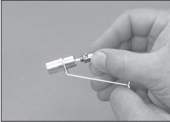
3.4 Load ST Connector into the shorter end of the 3M™ Universal Connector Holder.
