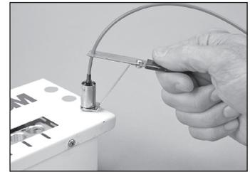
6.21 Rest the connector holder in one of the available cooling ports located on both sides of the oven. Let cool for three minutes.
