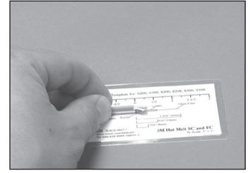
6.15 Check the final strip lengths and adjust if necessary.
