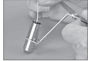
5.15 Feed the fiber into the back of the 3M Hot Melt Connector, until the buffer stops inside the connector.
