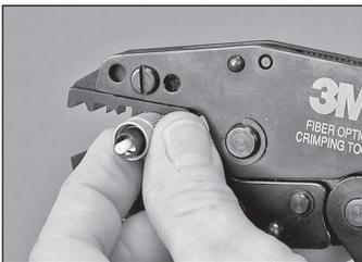
7.19 Once connector has cooled, remove from connector holder. Using the die labeled .190, crimp the large portion of the crimp ring onto the connector.
