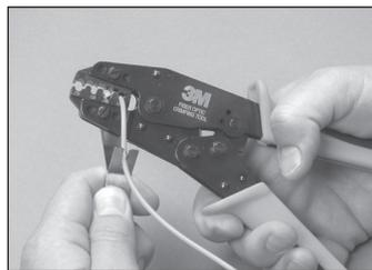
6.23 Secure the small portion of the crimp ring onto the jacket with the die labeled .137.
