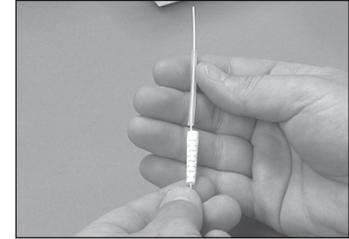
3.6 Place the strain relief boot and clear strain relief tube on the buffered fiber, as shown.
