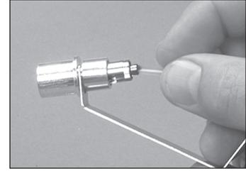
3.15 Slide the clear strain relief tube into the connector until it stops.
