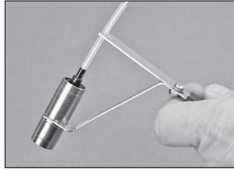
5.17 Push the buffered fiber into the cable retention feature until secure.
