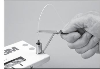
7.18 Rest the connector holder in one of the available cooling ports located on both sides of the oven. Let cool for three minutes.
