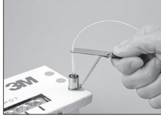
3.17 Rest the connector holder in one of the available cooling ports located on both sides of the oven. Let cool for three minutes.
