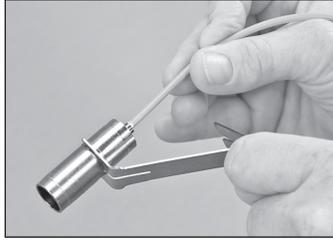
4.17 Feed the fiber into the back of the 3M Hot melt Connector, pushing until the Kevlar® fibers and jacket are secured inside the connector.
