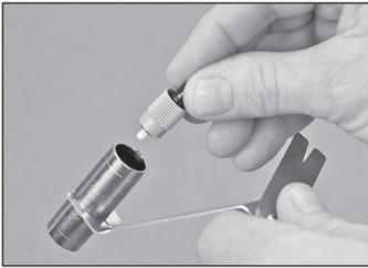
7.4 Load the FC Connector into the longer end of the 3M™ Universal Connector Holder.
