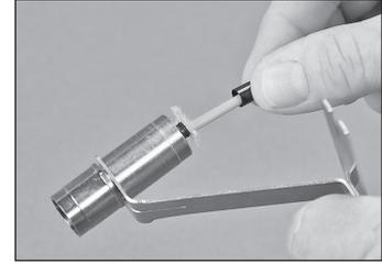
8.18 Feed the fiber into the back of the 3M Hot Melt Connector, pushing until the jacket stops on the connector. Flare the Kevlar® fibers equally around the buffered fiber.
