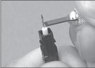
9.4 Score the fiber by gently sliding the blade across the fiber just above the bead of adhesive. Scoring means that you are making a small scratch on the outside of the fiber.
