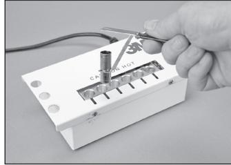
6.17 Remove the 3M™ Universal Connector Holder from the Hot Melt Oven by grasping the cool-touch handle.
