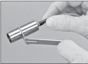
6.19 Slide the metal crimp ring onto the back of the connector, capturing the Kevlar® fibers.
