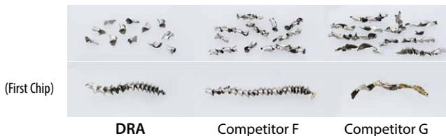
Cutting Conditions :  $V_c = 200$  sfm,  $f = 0.008$  ipr, Drilling Diameter 0.551"
