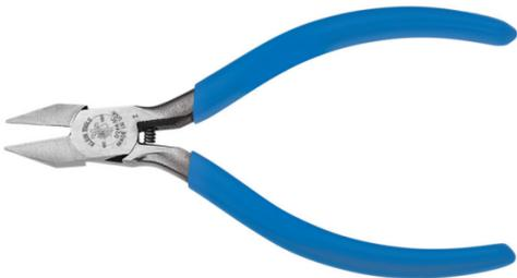
These Klein Tools 5-Inch, Electronics Pliers have a narrow jaw and hinge with a sharp pointed nose for precision in tight areas. These short jaw pliers have beveled standard cutting edges for perfectly flush cuts. They are made of US-made steel and are induction hardened with a spring assisted hot-riveted joint for a smooth action and long lasting durability.
