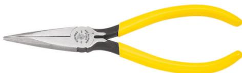
These Long-Nose pliers are spring-loaded for self-opening action. The slim head design works well in confined areas. Jaws are knurled for sure wrapping and looping of wire. Curved handles provide greater tool control while the joint is hot-riveted for smooth action and no handle wobble. Made of the finest U.S. steel alloy, they are forged, precision machined, hardened, and carefully tempered for maximum strength.
