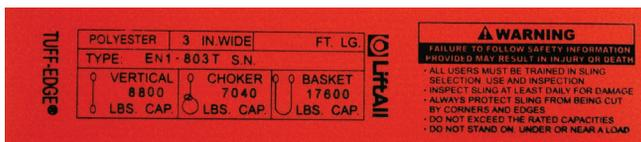
OSHA requires all web slings to show rated capacities and type of material. The *Lift-All Tuff-Tag* is made from an abrasion resistant polymer that will remain legible far longer than any leather or vinyl tags. In fact, *Tuff-Tags* will consistently outlast the useful life of slings.
