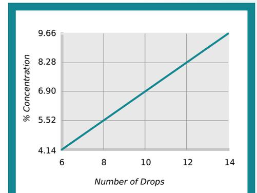
$\% \text{ Concentration} = \text{No. of Drops} \times \text{Titration Factor}$
