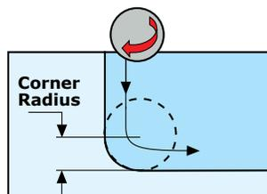
Ex: 1/4 tool, minimum corner radius to be generated is .1625.
