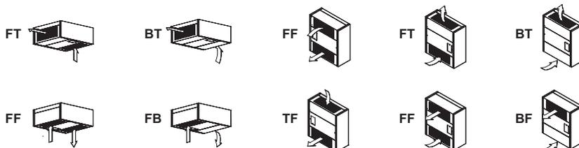
Several airflow configurations are possible and adaptable on-the-spot
