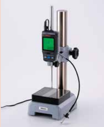
Application example using Digimatic Indicator ID-H.
