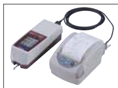
Example of the connection with SJ-210
