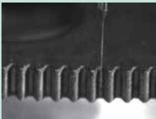
Measuring form of micro gear teeth
