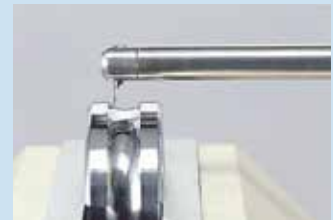
Inner/outer ring contour of a bearing
