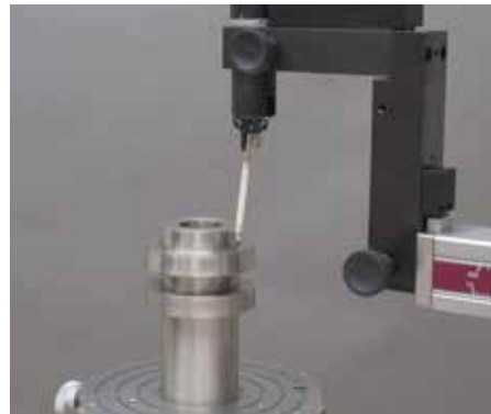
Spiral-mode cylinder measurement
