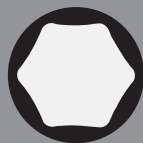
TORQUEPLUS™ 6 POINT SOCKET
