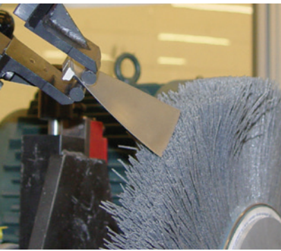
Deburring the tip of a turbine blade.
