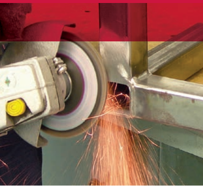
Grinding welds on a fabricated steel part.
