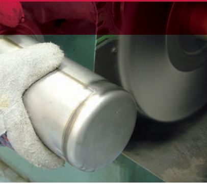
Removing heat discoloration from a stainless steel canister.
