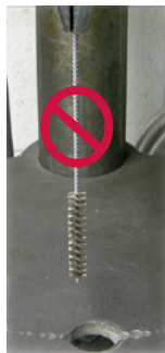
Incorrect Mounting in Chuck
