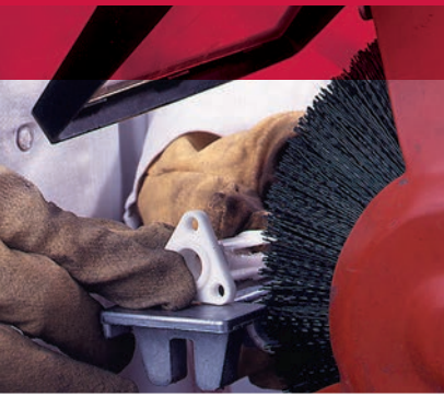
Deburring a plastic part using a nylon brush.
