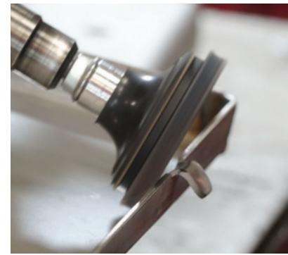
Edge chamfering a fabricated stainless component.
