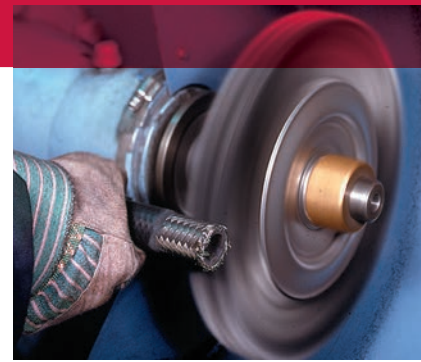
Removing rubber coating from a hydraulic hose.
