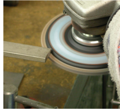
To trim backing, run against a sharp edge until desired backing diameter is achieved.
