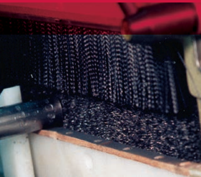
Straight strip brush used as a guard to prevent chips from flying.
