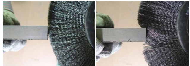
Correct Wire Tips Doing the Work
