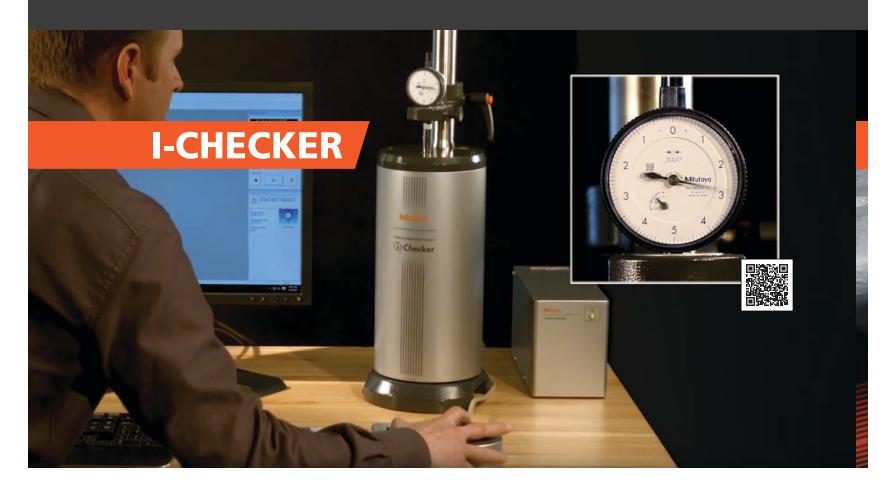
Inspect your indicators with Mitutoyo's I-Checker Instrument for efficient in-house calibration. The I-Checker can be used on various indicators such as Dial, digimatic and dial test. Also used for calibration of Bore gauges.
