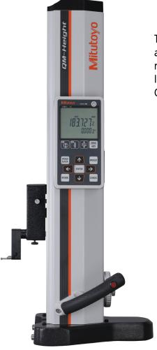
The QM-Height Series is a high-performance height gauge, with best-in-class accuracy  $\pm (2.4+2.1L/600)~\mu m$ , a built-in air suspension feature option for smooth movement, and an easy to view simple control panel. Click the View Product Information button below, to learn more about the benefits of purchasing the QM Height, now for a limited time only, 20% off!
