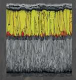
With Inveio<sup>®</sup>, every crystal in the alumina coating is lined up in the same direction, creating a strong barrier towards the cutting zone.
